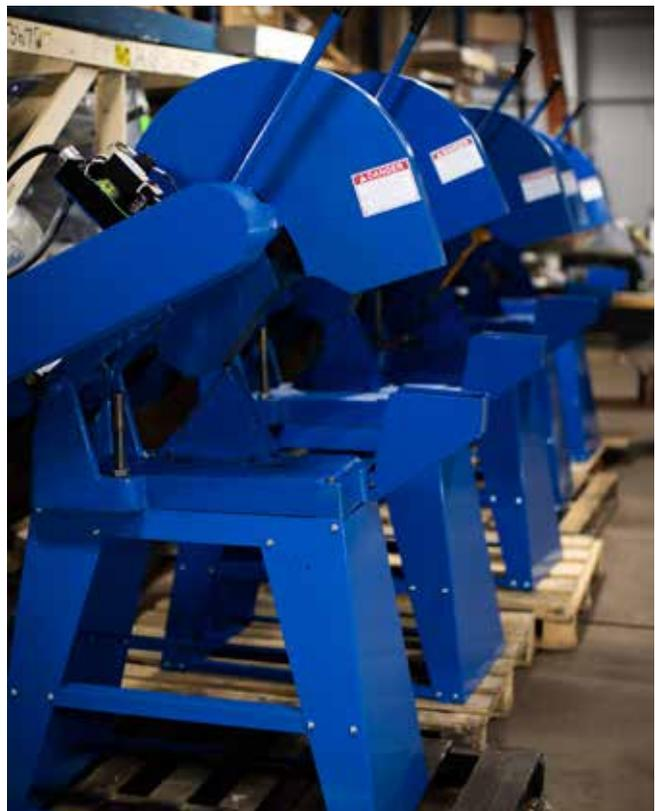
*The HYDM 2200. Built for cutting industrial hoses up to 10" in diameter.*
