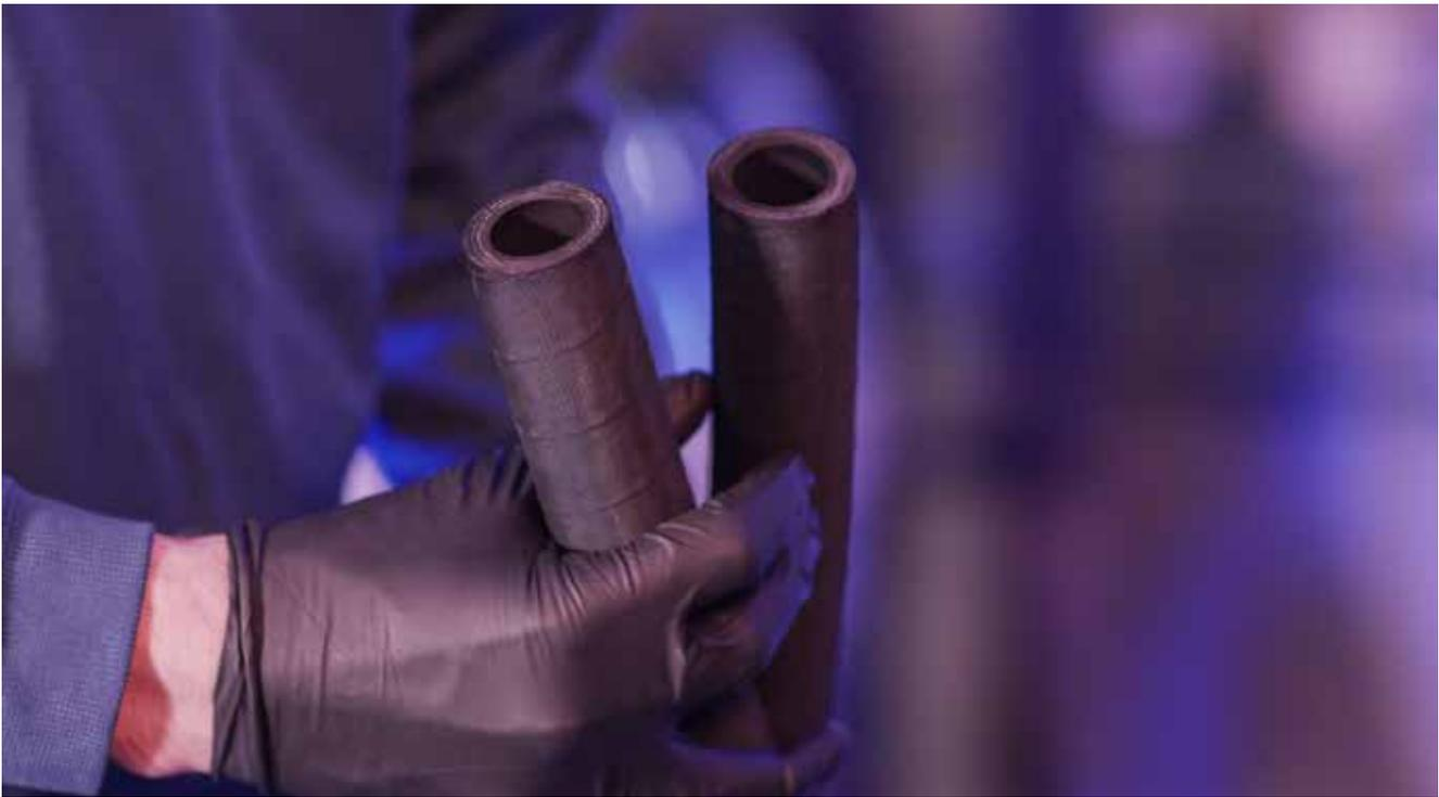
*The cleanliness and squareness of the cut obtained with a Specialty Saw system, allows for superior fitting assembly.*
