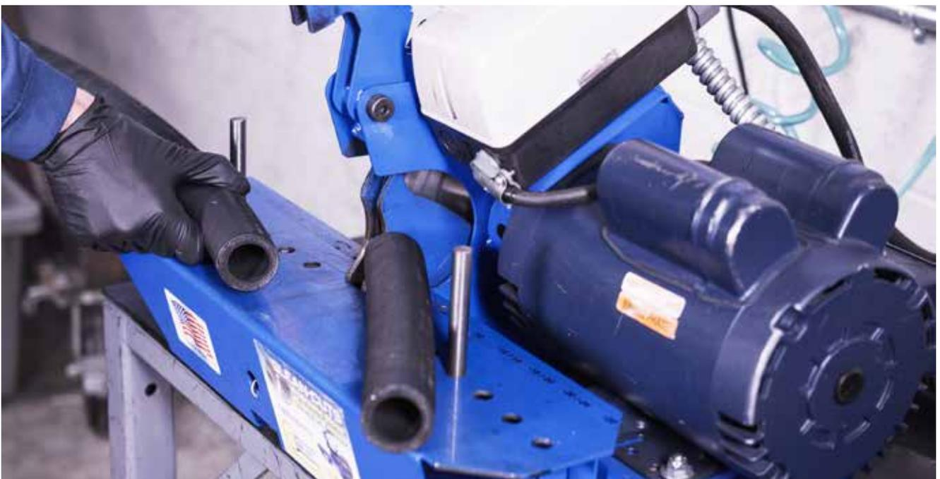
Specialty Saw's HYDM 100 in production at a hose distributor facility, seamlessly cutting an industrial hose with its Clean-Cuts™ technology.
