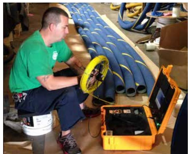
*Hose inspection at Montgomery Rubber & Gasket.*
